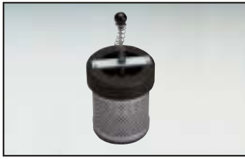
Protection valve. For safe lifts using fixed hooks/tools. Fitted between the lift tube and the vacuum head. Immediately eliminates the depression inside the lift tube, if the load is released inadvertently.
